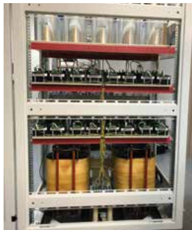
25kV dc PCS phase-leg prototype with 35kW power rating using 10kV SiC MOSFET.
