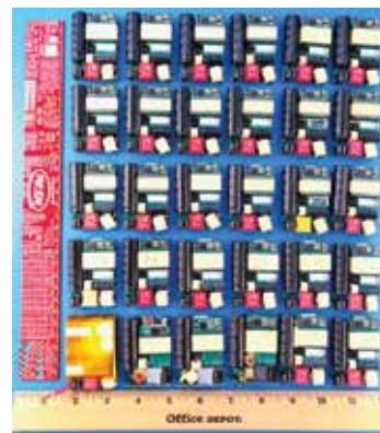
30 manufactured high density 500kHz GaN-based adapter units.
